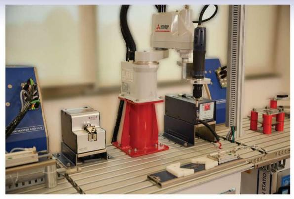
The process in this setup includes automatic dispensing of two different jobs, press assembly of dispensed jobs, bolt assembly of assembled jobs and vision inspection end product.
