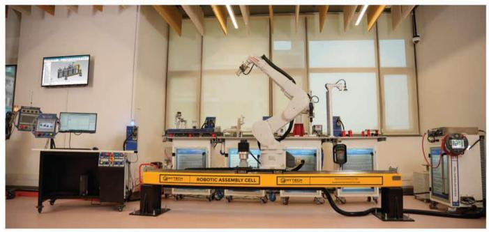
Hytech Didactic integrated assembly cell is an integrated robotic cell which provides users with hands on experience on robotic bolt assembly process. This cell is integrated with PLC – HMI and SCADA. Four automation stations are provided to carry out assembly process along with vision inspection. This cell includes an industrial 7 axes robot with industrial linear gantry axis and a four axes SCARA Robot with a DC Nut runner attachment.
