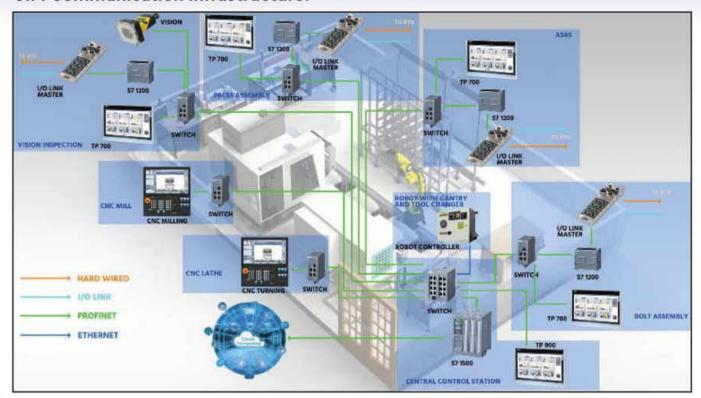
Stations in CIM are provided with I/O Link masters as well as individual PLCs and HMIs which enables them to be programmed and operated individually. User can integrate these stations with central SCADA system as well as central PLC in CCU.
