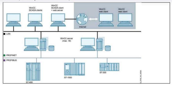
The SCADA acronym stands for Supervisory Control and Data Acquisition.
