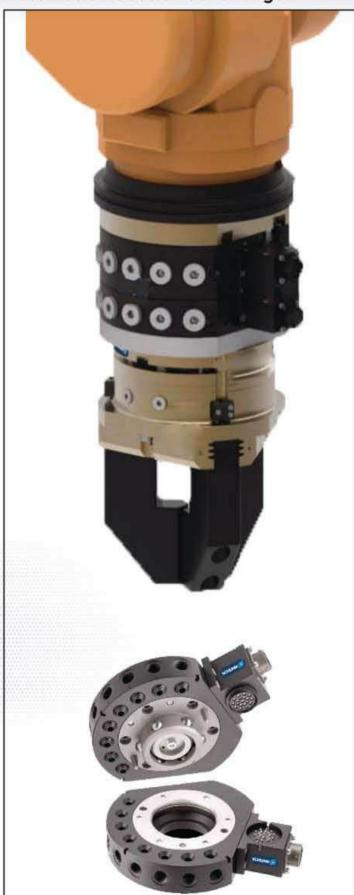
Automatic exchange of the end effector increases the flexibility of robot.
